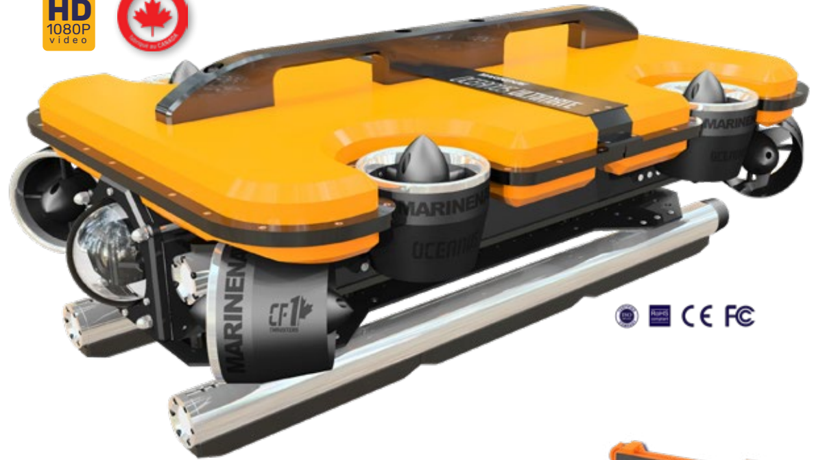
Oceanus Ultimate ROV system includes Ultimate ROV, 18.5-inch topside control case and Oceanus hand controller
